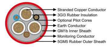
Conductors: Flexible stranded copper conductor, class 5 according to DIN VDE 0295.
